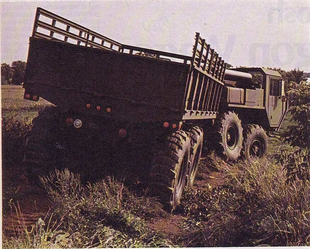
This photo taken from the rear permits the reader to appreciate the movement of the frame and the attitude angle on rough ground.
