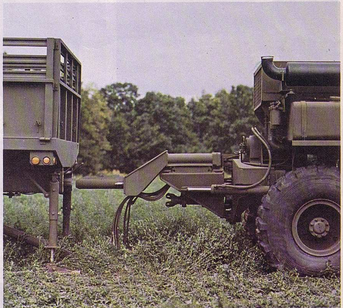
Detail of the articulation joint. Note one of the steering cylinders in the note foreground the transmission shaft and the electrical and pneumatic cables.
